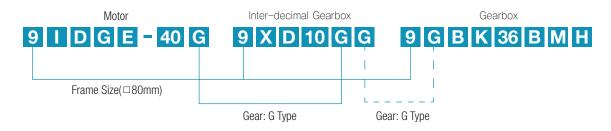
• When attaching inter-decimal Gearbox, the output shaft type of the motor is always G Type.
