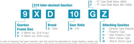
Inter-decimal Gearbox with general Gearbox. And please be advised that in this case only revolution speed of output shaft will reduce by 10:1 without increasing of maximum permissible torque.
