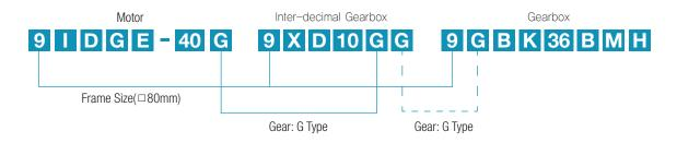
• When attaching inter-decimal Gearbox, the output shaft type of the motor is always G Type. For example, when using P/H/W/WH type Gearbox, only the gear type of inter-decimal Gearbox is identical with attached Gearbox and the output shaft type of the motor is G type. (Refer to the scheme below.)
